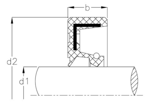
$\begin{array}{ll} b & = 10 \\ d1 & = 70 \\ d2 & = 100 \\ Material = NBR \end{array}$
